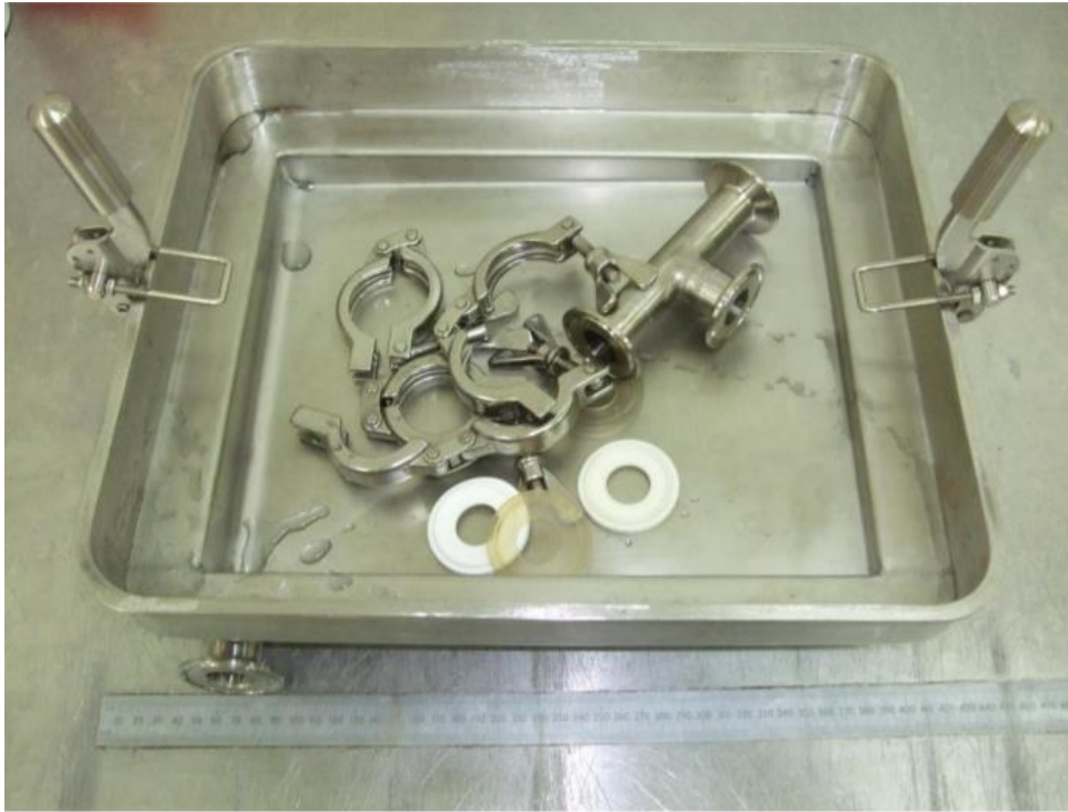
Figure 2: The hopper tray is washed and placed back into the hopper during drying.
